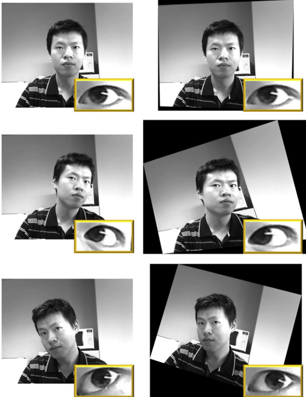
Fig. 6. Eye image rectification. By using projective transformation, captured images (left) are rectified (right) so that eye regions (shown in small rectangles) can be better aligned with each other.
